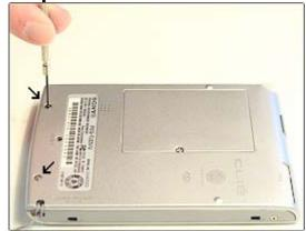
Remove the two "Y Head" three pointed screws below the label on the back of the device, as shown, using the included mini flathead screwdriver. (Your tools may look different than the picture shown.) You can also use a "Y Head" screwdriver if you have one. Set the screws aside for reassembly.
